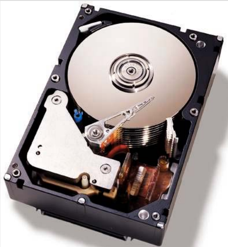
Top view of a 36 GB, 10,000 RPM, IBM SCSI server hard disk, with its top cover removed.
